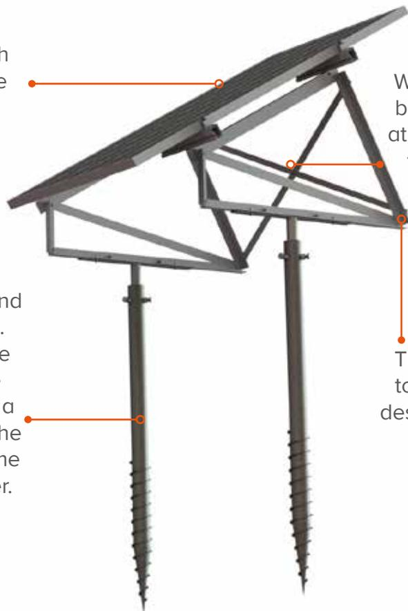
Wind bracing is added to the back of the elevation frames at certain intervals to stabilise the system against lateral movement.
